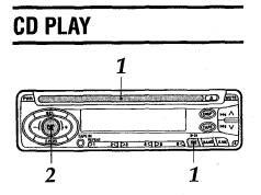
Insert a disc with the labeled side upward to start CD play.
